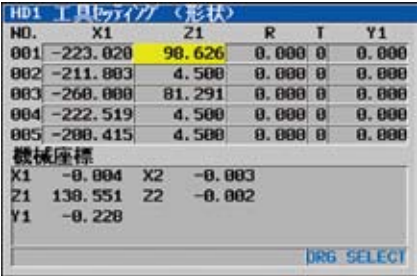
Tool setting Used to measure geometry offsets. It can also be used for tool mounting support, to ensure that the overhang of all tools is fixed at a constant value.
